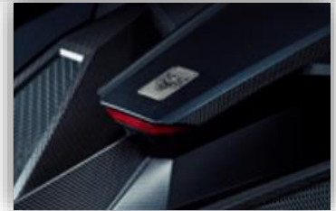
Graphene enhanced prepreg used by W Motors
