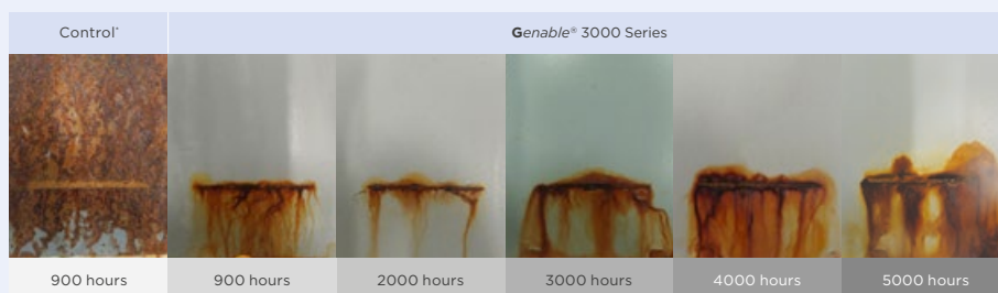
*Control is an in-house primer typical of a standard industrial C3 zinc phosphate based system
