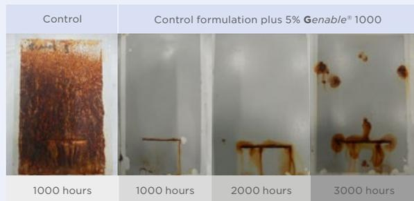
Substrate: SA 2.5 Sandblasted Steel
