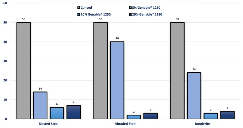
• With each loading of graphene, a significant reduction in the levels of creep was recorded compared to the control
