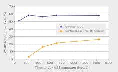
50-60 micron DFT, comparative water uptake under NSS exposure
