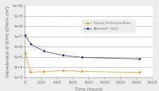
50-60 micron DFT, impedance measurements carried out at 10 day intervals.
