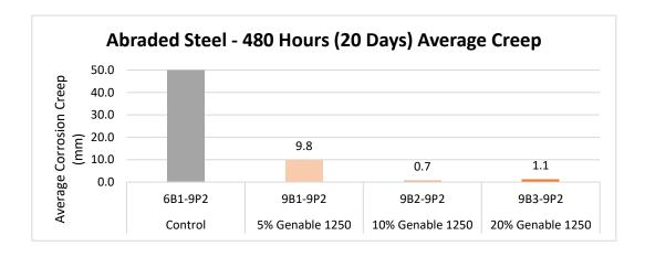
**Note**: Except for the 480-hour assessment of the coated Blasted Steel control panel all of the other control panels at both 480 hours and 1000 hours testing had substantial levels of corrosion emanating from the scribe and/or a complete failure in terms of corrosion. These panels have been denoted as having an average creep corrosion of 50mm to aid pictorial representation in the graphs above.
