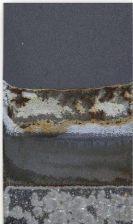
Complete coating failure of glass flake control system
